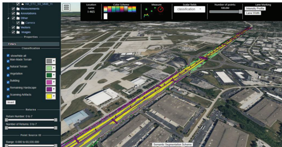
Figure 4.7 Example of visualizing semantic segmentation results: man-made terrain is colored in grey, natural terrain is displayed in light green, vegetation is marked in dark green, buildings are colored in pink, the remaining hardscape is depicted as purple, and scanning artifacts are yellow.
