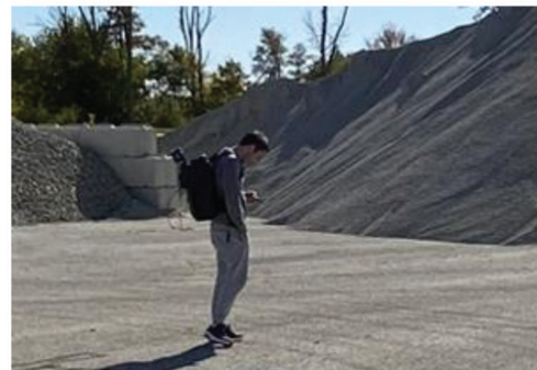
Figure 6.6 Illustration of (a) study site in Greensburg, IN, showing the stockpile enclosed by the blue rectangle, (b) corresponding stockpile for volume estimation, (c) 3D stockpile scanned by UAV showing the volume estimate, and (d) 3D stockpile scanned by Backpack system while displaying the volume estimate.
