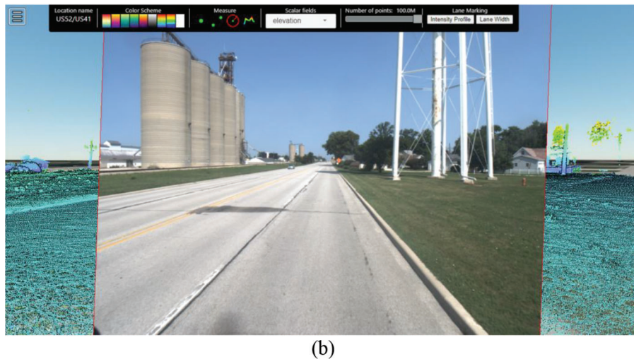
Figure 4.6 An illustration of visualizing geo-tagged imagery showing (a) a selected geo-tagged imagery, and (b) visualization result of the superimposed on LiDAR data in the web portal.
