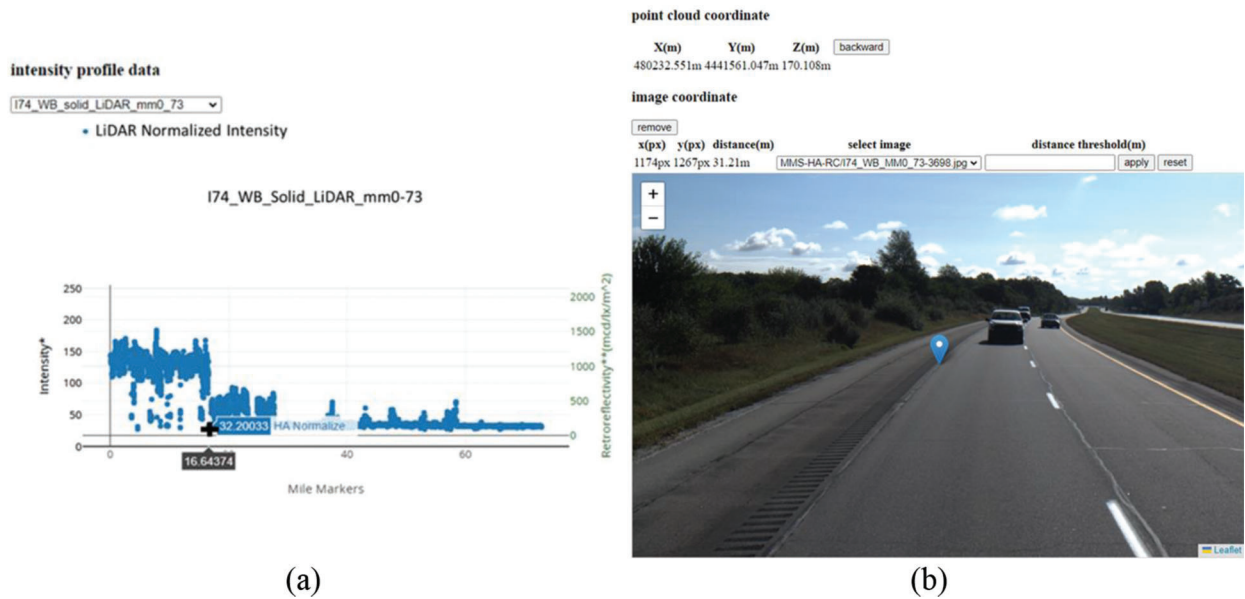
Figure 4.14 Illustration of (a) intensity profile with a selected point showing low intensity, and (b) corresponding image including the same point in the web portal.
