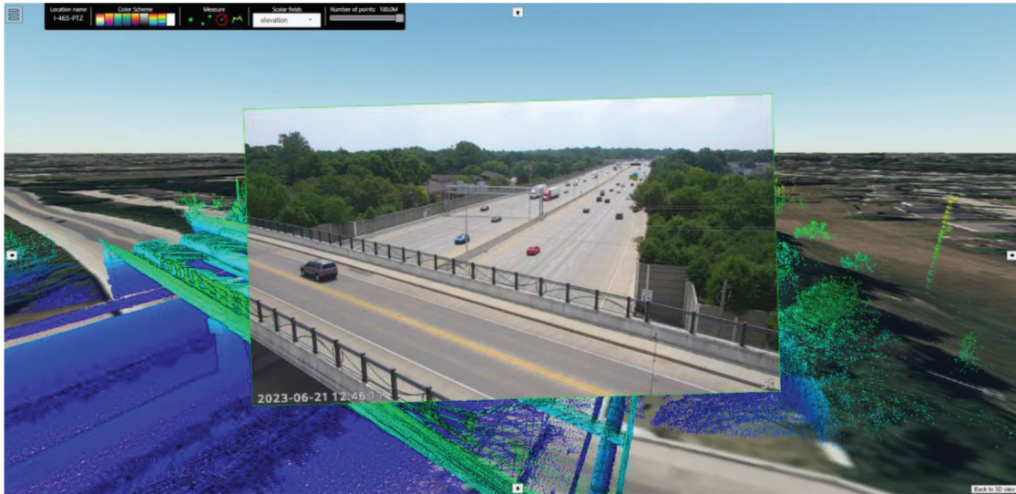
Figure 6.3 Illustration of calibrated image from PTZ camera super-imposed on LiDAR data visualized in the web portal.
