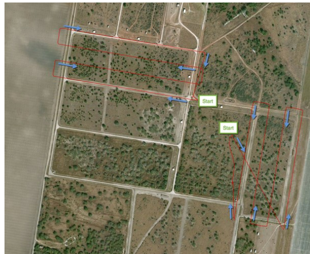
Fig. 1. Experimental pastures at the USDA-ARS Cattle Fever Tick Research Laboratory, Moore Airbase, Edinburg, TX. UAV flying path design (Solid red lines indicate autonomous flight path, blue arrows indicate flying direction, and green squares indicate ground control station where UAV was launched and landed after the mission.)
