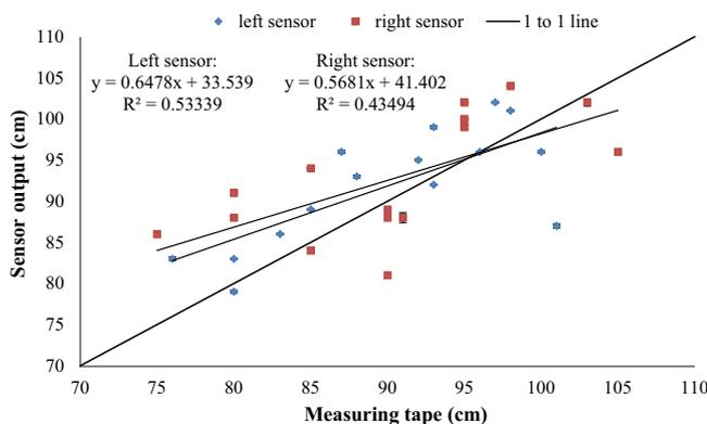
Fig. 2. Comparisons of Left and Right SR50A cotton height measurements with a tape.
