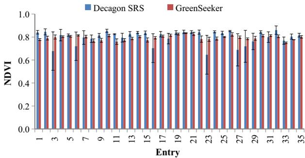
Fig. 5. Average Normalized Difference Vegetation Index (NDVI) measurements taken for cotton plants with a Decagon SRS and a GreenSeeker sensor. Plots contained approximately 90 plants. Bars represent  $\pm$  standard error of measurements.
