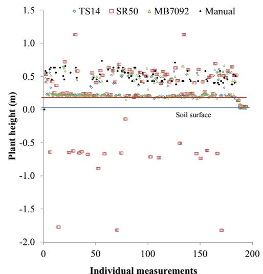
Fig. 3. Comparisons of three sonic ranging sensors with manual measurements in a peppercow. Weslaco, TX, 2016. The black dots represent the height of each individual plant in the row. Red line represent the elevated bed in which pepper plants were planted.
