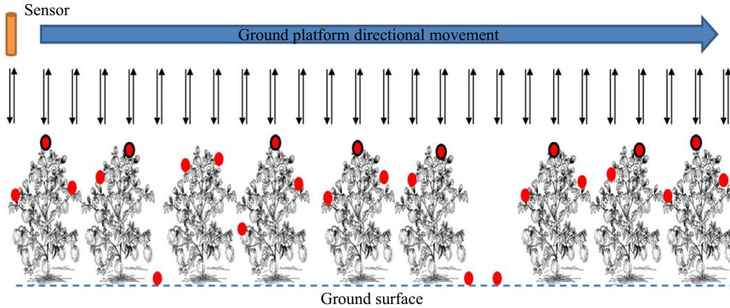
Fig. 4. Simulation of the movement of the platform and collection of ultrasound data. The red dots with black borders indicate the real, thus desired height of the plant.
