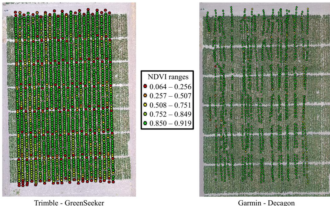
Fig. 6. Differences in GPS receiver accuracy. Normalized Difference Vegetation Index (NDVI) values are shown for reference. Data collected on 6/26/2015 at the Texas A&M AgriLife Research and Extension Center, Corpus Christi, TX. Red and green dots represent lowest and highest NDVI values, respectively.
