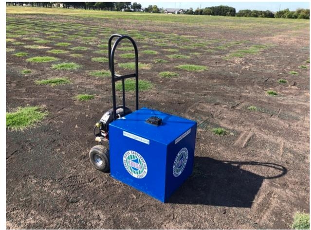
Fig. 3. The light-box was used to mount a camera for the collection of ground imagery data.
